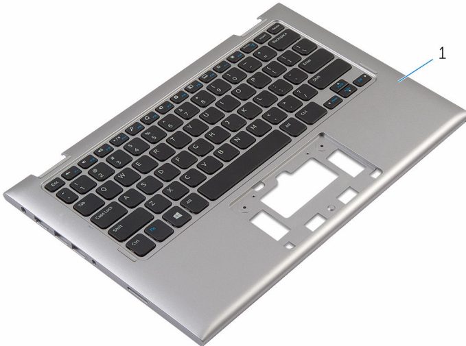
1 palm rest and keyboard assembly
